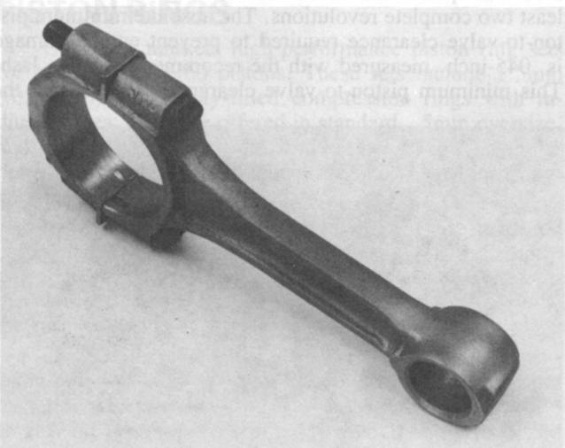
Figure 34 — Grind off forging marks and shotpeen beam to improve durability of production rods used in high-performance V6s.
