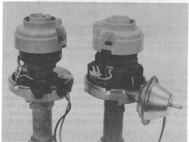
Figure 89 — S-10 distributor has vacuum cannister and magnetic pickup (right). Eliminate vacuum advance and connect pickup directly to Chevrolet heavy-duty ignition box for off-road racing.
