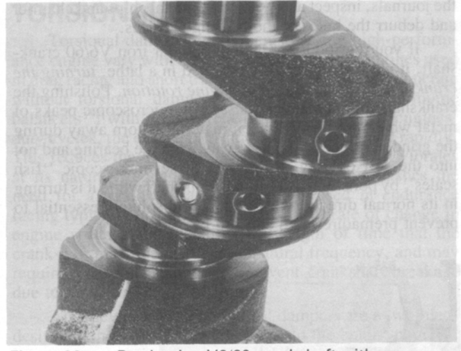
Figure 23 — Production V6/60 crankshaft with cross-drilled main bearing journals.
