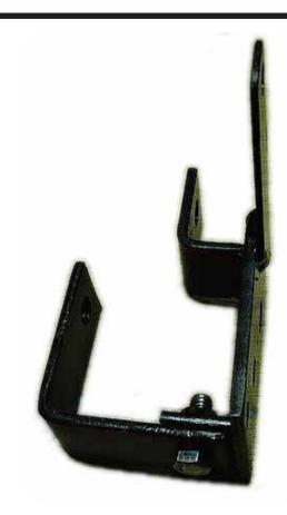
The bracket consists of two pieces of 1/8" steel bolted together. The main piece is flat plate with welded-on alternator mounting arm and "L" shaped mounting leg. The second piece is a larger "L" leg that bolts to a mounting flange on the bottom of the main piece. Both pieces bolt to the front of the engine at the mount.
