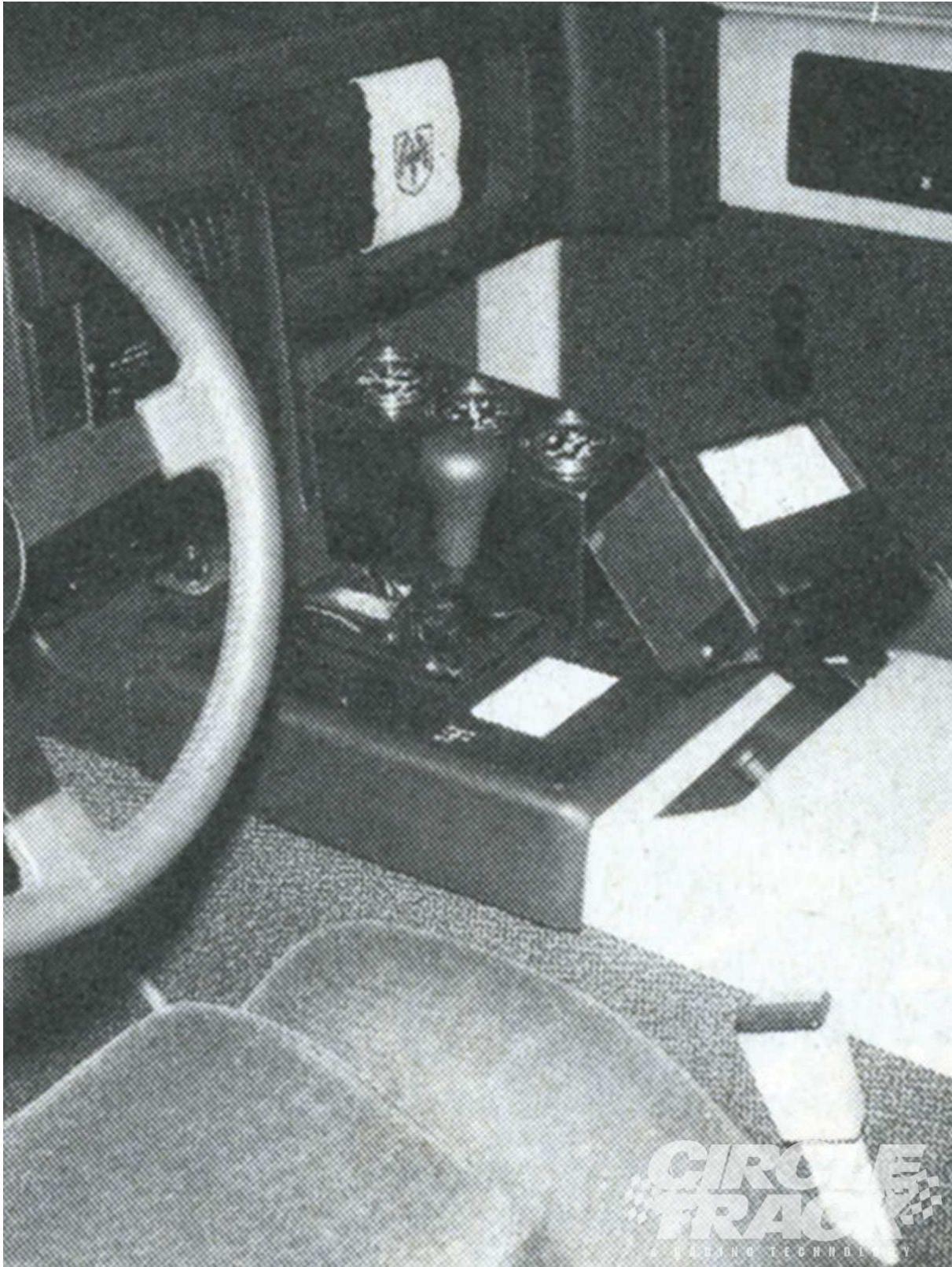
Added to the interior of the Fiero were manifold vacuum/boost, oil pressure, and water temperature gauges in addition to a tachometer. Not shown on the floor were exhaust temperature and fuel flow meters.
